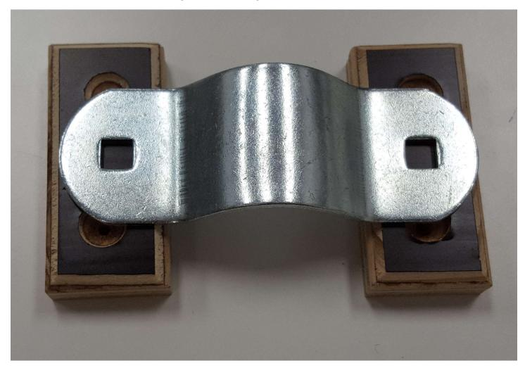
This photo shows the suggested method of mounting the bracket on two wooden blocks. There should be pilot holes drilled into the center of the blocks (not shown in this picture).
