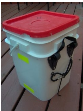
Illustration 1: MEC attachment system – hangers on top and J-hook/shock cord on bottom.
